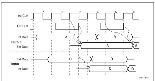
Figure 16-18. Processor 2/5 Bus Internal/External Data Movement
